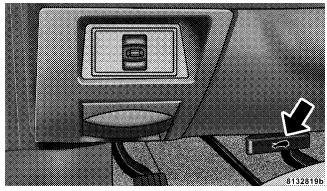
Then push the safety latch lever to the right. It is located between the grille openings left of the center.
